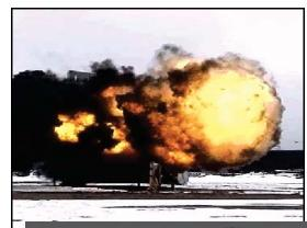
Controlled demonstration showing the explosive potential of 52 lbs. (approx. 5-gallon pail) of PRB coal dust.
